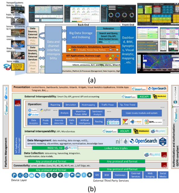
Figure 4: Overview of the Snap4City functional (a) and technical (b) architecture.
