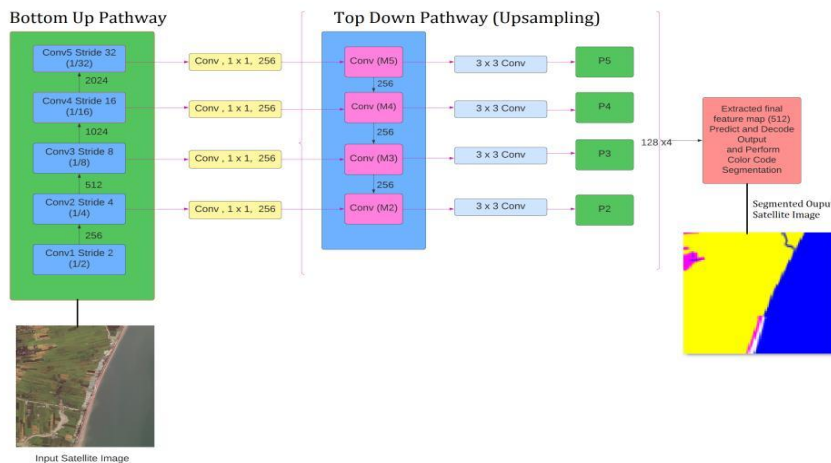
Figure 4: FPN Segmentation Model Architecture
