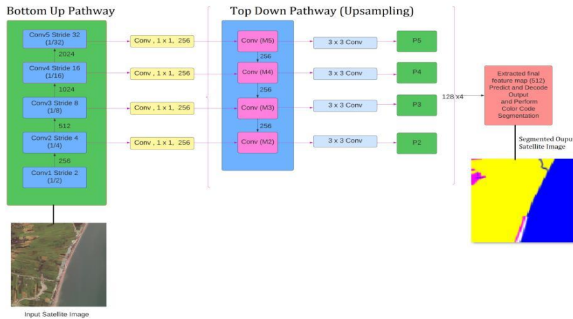
Figure 4: FPN Segmentation Model Architecture
