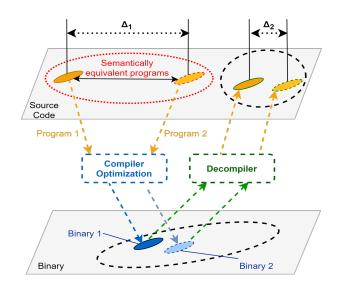
Fig. 1:  $\triangle_1$  represents the distance between the vector representations of two semantically similar source code.  $\triangle_2$  represents the distance between the vector representations of the decompiled binaries of the source code.
