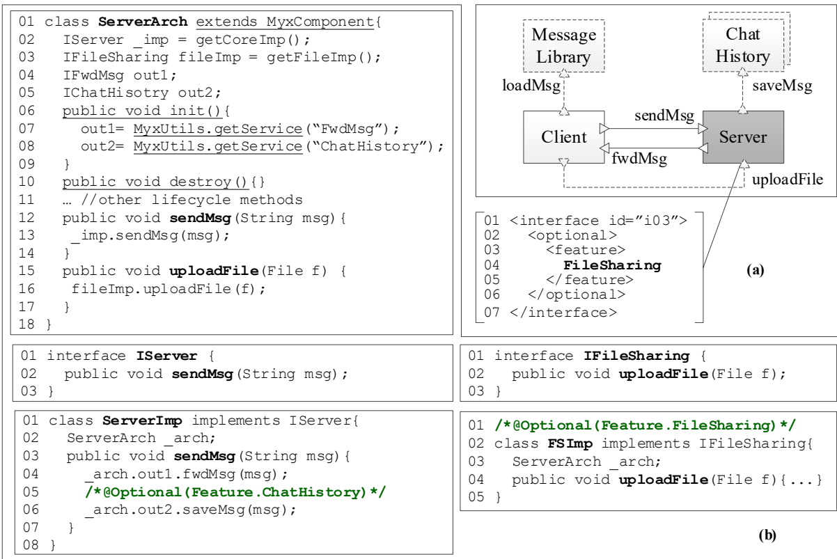
Fig. 3. (a) Architecture example of a chat application; (b) Code example of Component Server .
