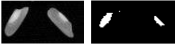
Figure 6: The left sub-figure shows the original image, while the right sub-figure shows the separated chalky with Eq.(9).
