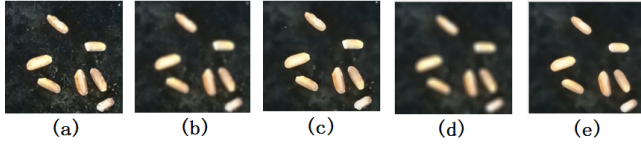
Figure 3: (a) indicates the original sample. (b) indicates the filtered sample with Gaussian filter [1]. (c) indicates the filtered sample with Bilateral filter [15]. The filtered sample in sub-figure (d) is from the Average filter while that in sub-figure (e) is from the Median filter. From the results, we can see that the denoised result from Bilateral filter is better than others.
