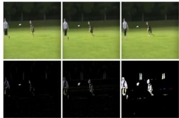
Figure 4: The first three frames are adjacent frames, the fourth one is the corresponding residual frame, the fifth one is the residual frame after the absolute value, and the sixth one is a binarization of the fourth one.
