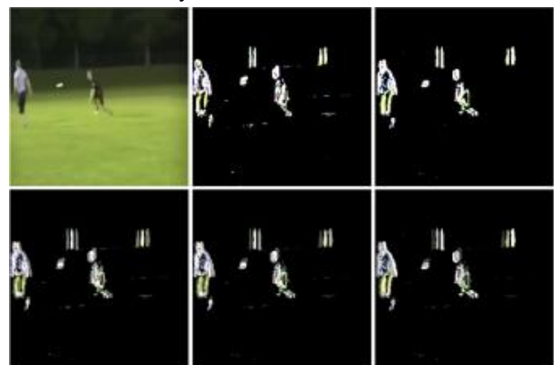
Figure 2: Motion Detection. The second and third frames are the two consecutive temporal differences before the first RGB frame. The fourth frame is (df1 + df2) , the fifth is (2 * df2 + df1) , and the sixth is the DRF, where df1 is Frame 2, and df2 is Frame 3.
