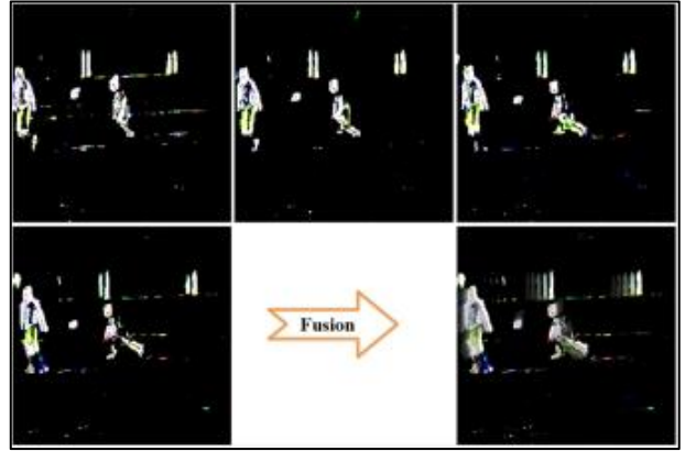
Figure 6: The first four pictures are continuous residual frames after binarization, and the last one is the DRF fused by the first four.
