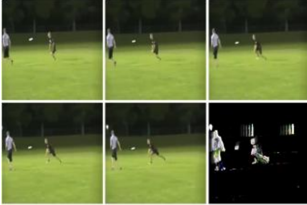
Figure 1: The first 5 frames are consecutive frames in the video, and the sixth frame is the corresponding DRF.
